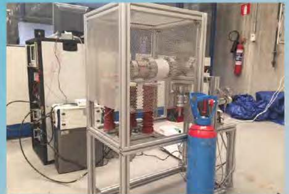
Figure 1: The low-current compact ion source designed and built by GAUDEE.
